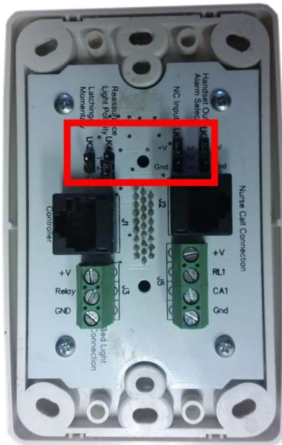
Figure 7: Location of the jumper shunts. They do not need to be changed.
